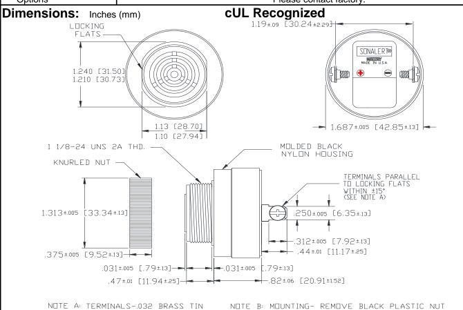
PLATED, TAPPED FOR #6-32 SCREW. TWO #6-32 NICKEL PLATED BRASS SCREWS INCLUDED. WILL ACCEPT 1/4"
