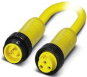
Power cable, 3-position, PVC, yellow, Plug straight 7/8"-16UNF, A - standard, on Socket straight 7/8"-16UNF, A - standard, cable length: 10 m
