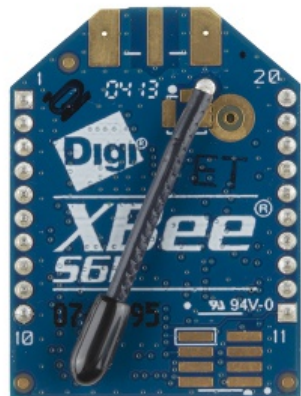
XBee WiFi modules with PCB antenna (left) and whip antenna (right). No external antenna needed!
