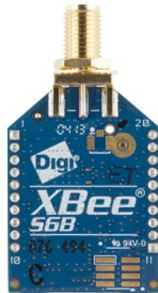
XBee WiFi modules with a U.FL (left) and SMA (right) antenna connector.
